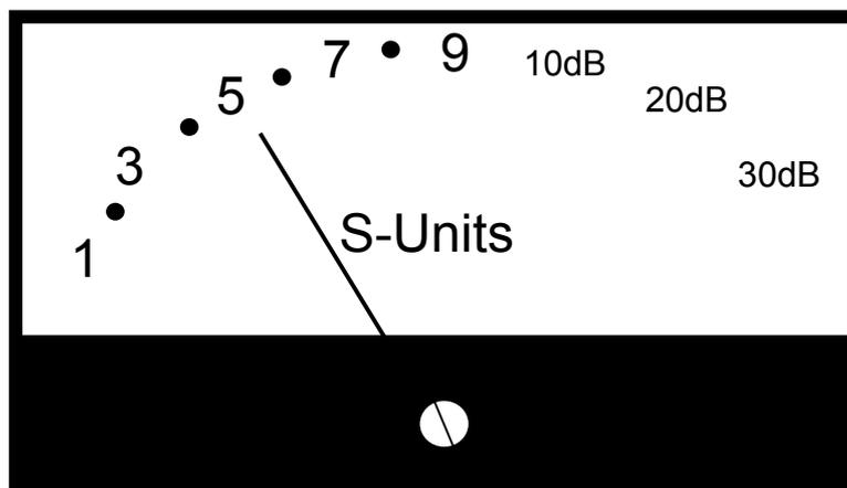
S-Meter showing a reading of S5
