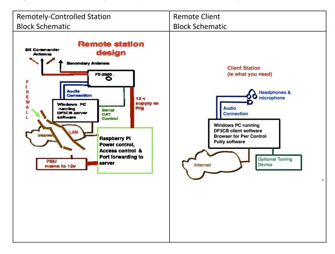
The access control run by the Raspberry Pi is key. Once you are logged onto the Raspberry Pi (using Putty software), you will then be able to
