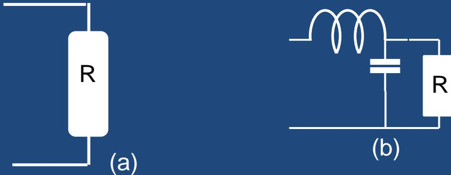
Now elaborate the load by adding a small inductance in series and a small capacitance in parallel (b). If the capacitance really is small, its reactance  $X_c$  will be much greater than  $R$
