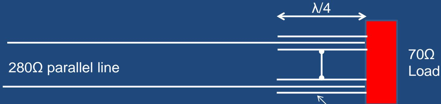
Suppose we wished to connect a 70Ω load to a 280Ω parallel wire feeder without reflection from the junction.
