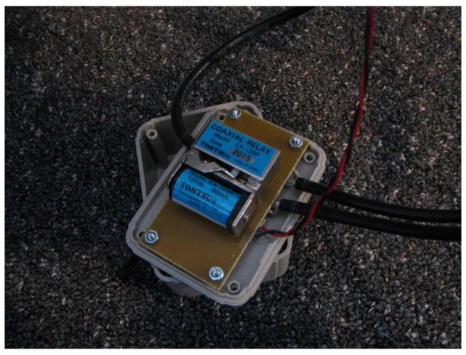
Each relay is mounted on a small piece of PCB using the island technique for direct connection to flying leads. The outside of the case is marked with the relay number and the normally closed connection. The relay number has no electrical significance but is useful for tying up with the patching diagram.
