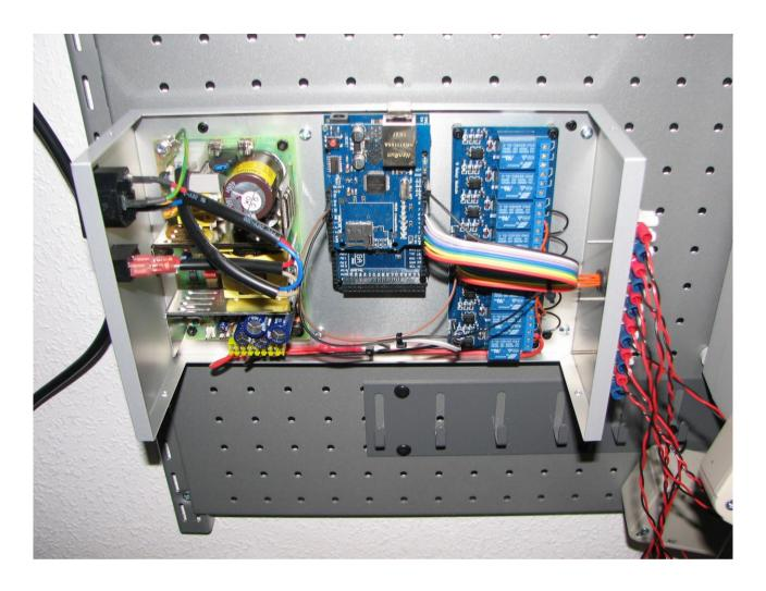
The enclosure is a simple aluminium box which provides reasonable screening.
