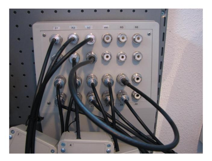
This is a pretty simple arrangement with the antenna ports at the bottom and the radio ports at the top. These are simply wired to their corresponding patch sockets with short pieces of RG58. The enclosure is an ABS console type form factor box. I didn't at this point want to common up the earth side, hence ABS.
